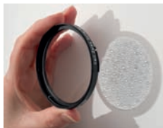
Small moulded lenses on surface of soft focus filter can be seen in its shadow.
