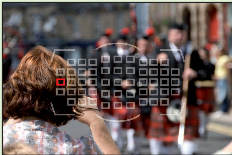
Pictured here is a representation of the viewfinder using the Nikon 51-point AF system showing one user-selected sensor in Single-point AF mode.
