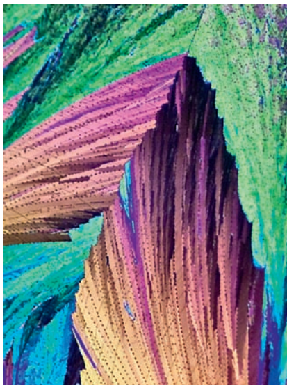
Pictured here are paracetamol crystals in polarised light x40 imaged with a Kodak Professional DSC 520 (Canon mount) on a Brunel BMS trinocular zoom stereomicroscope.
