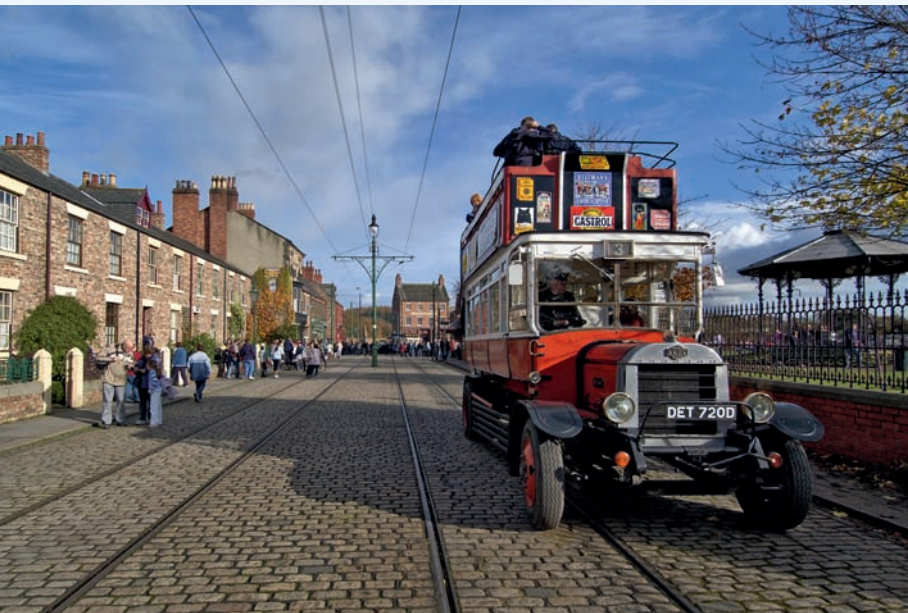
An open-air museum street scene showing the strong convergence of lines and dramatically receding background; this was taken with the equivalent of an 18mm super-wide-angle lens with a 90° angle of view.
